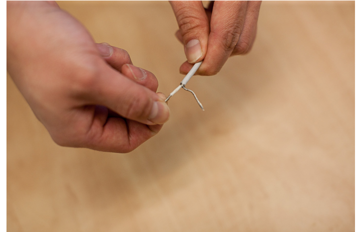
STEP 17: Twist the center wire strands into a single twisted strand.
