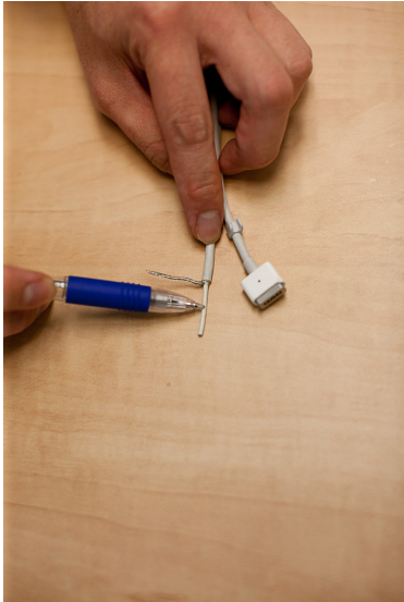
STEP 15: Mark the halfway point on the inner tubing.
