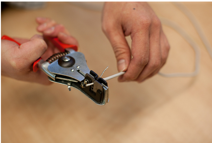
STEP 16: Align the 2 nd smallest hole with the pen mark made in STEP 15. Strip off the inner tubing to reveal the center wire strands.
