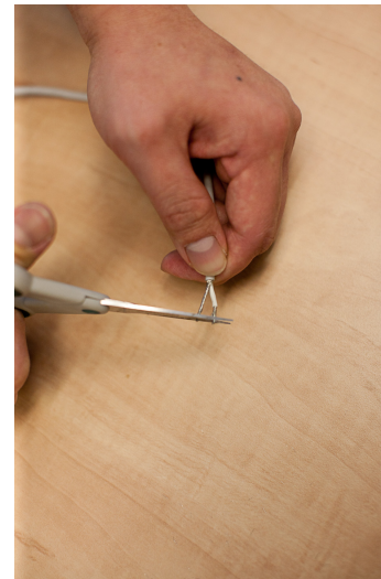
STEP 17: Twist the center wire strands into a single twisted strand.
